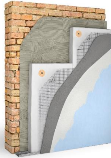
Layered scheme for exterior insulated sheathing
